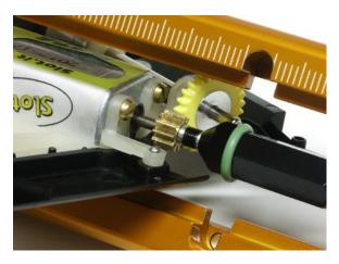
7. Press the pinion in place and remove tool. Done!
