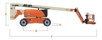
Platform Width 36-in / 0.91-m B. Platform Length 96-in / 2.44-m Machine Width C. 8-ft 1.5-in / 2.48-m Tailswing 2-ft 5-in / 74-cm D. E. Machine Height 9-ft 9.1-in / 2.97-m F. Machine Length 36-ft 9.9-in / 11.22-m G. Wheelbase 10-ft / 3.05-m **Ground Clearance** 11-in / 28-cm
