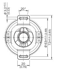
General tolerances according to DIN ISO 2768-mk Cable diameter = 5.6 mm +/- 0.2 mm bend radius = 30 mm
