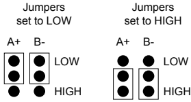
Figure 3: Setting the A+ and B- jumpers
