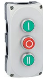
Grey control station LPZP3A8 complete with green flush pushbutton "i" LPCB1113 1NO, red extended pushbutton "o" LPCB2104 1NC and green flush pushbutton "ii" LPCB1123 1NO LPZP3B8903
