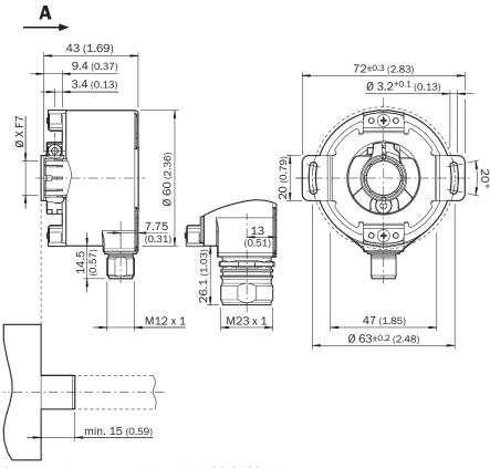
General tolerances according to DIN ISO 2768-mk ① Cable diameter = 5.6 mm +/- 0.2 mm bend radius = 30 mm
