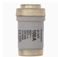
Cartouche fusible, Basse tension, 100 A, AC 400 V, 50 kA, D03, gL/gG, IEC, lent
