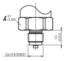
Housing with circular connector M12 x 1, IP67
