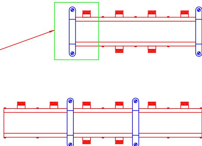
Recommended positions of the wall fixing set for an easy installation of the distributor.
