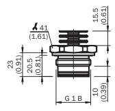
Housing with L-connector (DIN EN 175301-803 A)
