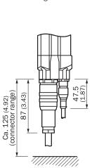
Cable socket M26 with crimp contacts (for DIN 43651, left) and cable plug M12 with cable (right, only on receiver)
