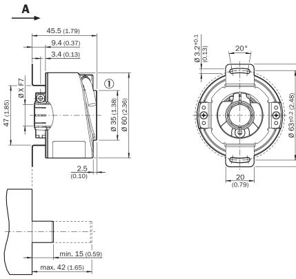
General tolerances according to DIN ISO 2768-mk (1) Cable diameter = 5.6 mm +/- 0.2 mm bend radius = 30 mm
