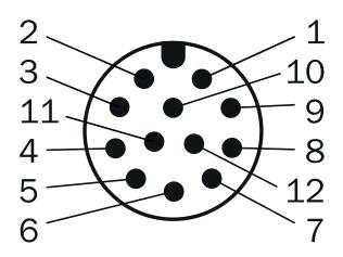
M12, 12-pin male connector, A-coded
