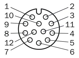
M12, 12-pin female connector, A-coded (I/O)
