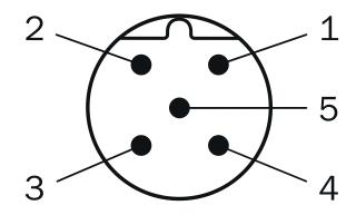
Male connector M12, 5-pin, A-coded
