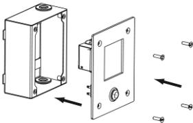
Refit the frame + diffuser assembly using a suitable screwdriver fitted with the **98000004** special bit.
