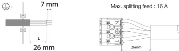
The cable must be prepared as per the diagrams. The conductors must be stripped for a length of 7mm. Respect the polarity.
