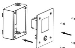
Remove the frame + diffuser assembly using a suitable screwdriver fitted with the 98000004 special bit
