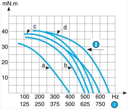
Inertia of measuring chain: 2,2 g.cm2 a = constant voltage controller with Rs (resistance in series) = 0 b = constant voltage controller with Rs (resistance in series) = R motor c = constant voltage controller with Rs (resistance in series) = 3R motor The measurements are made with full stepping, 2-phases energised.
