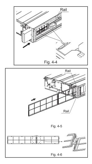
4.Insert the filter that was removed in step 3-1 above along the top and bottom rails.(Fig. 4-5) When using the PAC-KE93, 94, or 95PTB-E, join the two filters before inserting them. (Fig. 4-6)
