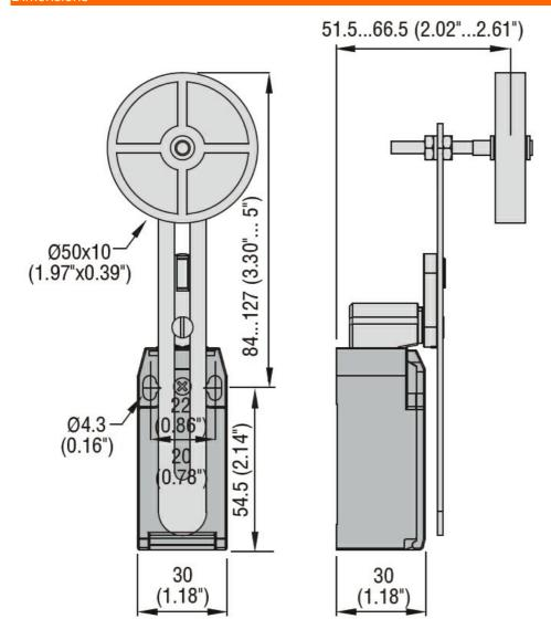
LIMIT SWITCH, K SERIES, ADJUSTABLE ROLLER LEVER, 1 BOTTOM CABLE ENTRY.
