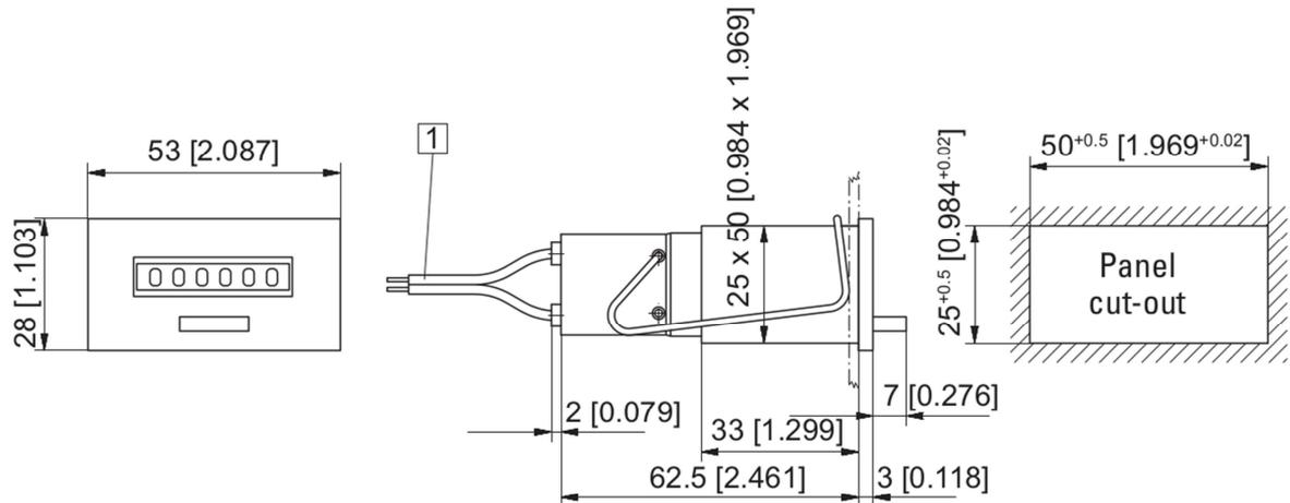
1 Connection cable, 2 x 0.5 mm<sup>2</sup> [AWG20], NYFAZ, 0.5 m [1.64'] long
