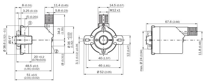
① Measuring point for operating temperature
