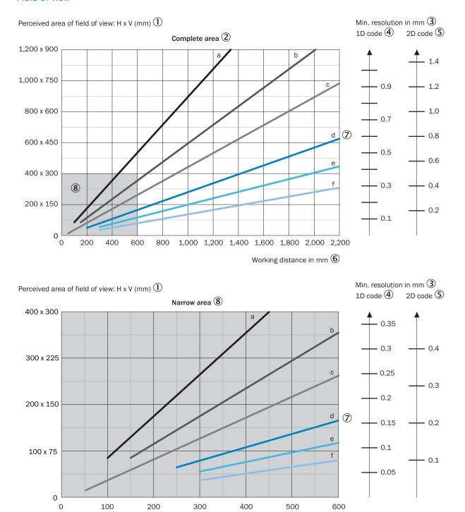
For S-mount and standard C-mount lenses, spacer rings are needed for working distances shorter than approximately 10 times the focal length. For compact C-mount lenses, spacer rings are not needed, but the built-in illumination cannot be used for distances shorter than 300 mm.
