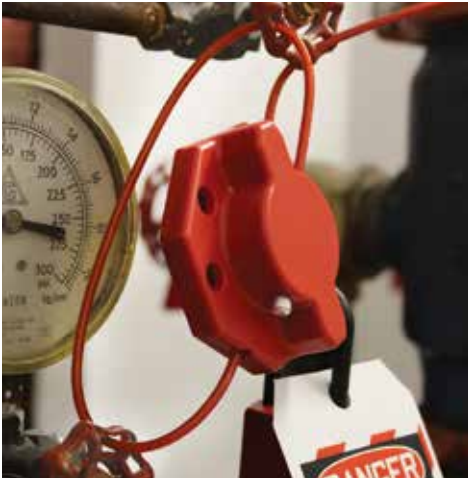
Turn the hasp halves to cinch cable.
