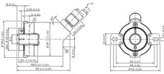
Non-tolerated dimensions according to DIN-ISO 2768-mk
