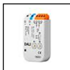
S.2492 Signal converter from DALI to VIRTUAL MIDNIGHT. Compact control IP20 module for automatic power reduction / brightness reduction for night-time. The device has an integrated bus supply (20mA) for up to 7 DALI luminaires. Possibility to extend up to max. 64 luminaires through the DALI Expander (S.2494). 2 operating modes are supported: - Operating mode B1: power reduction through mains phase or control phase; - Operating mode B2: power reduction using virtual midnight calculation. All necessary settings can be made using rotary and slide switches. The device must be located before the DALI luminaire inside an electrical cabinet / waterbox / junction box.
