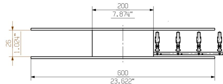
For the mounting of PCBs, it should be noted that the rated data given in the catalogue relates only to the connection elements. The necessary creepage and clearance paths must be observed in connection with the respective applicant in accordance to VDE 0110. The current-carrying capacity and pitch tolerance is to be determined according to DIN IEC 326 part 3 very fine.
