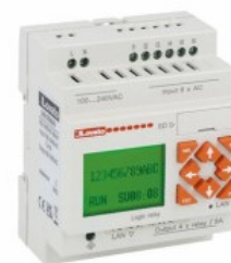
Micro PLC - Base module with built-in Ethernet port LRK10RA240 100...240VAC Nr. 6 digital Nr. 4 relay 10 (6 inputs + 4 outputs) up to 34 with LRE modules
