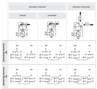
$<sup>\</sup>frac{1}{\mathbf{P}}$  Positive action N/C locking monitoring contact
