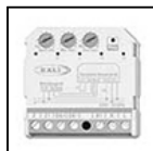
S.2490 Signal converter from PUSH DIM to DALI2 Features DALI-2 dimming (1-100%). Control unit for the conversion from push button to DALI-2 interface. Allowed powering up to 35 DALI-2 interface in BROADCAST. Input current typ. 70 Ma - max. 110 Ma. Application in installation boxes. Light regulation 1-100% by means of PUSH: - a short push to turn on and off; - a longer push to increase or decrease light intensity. Dimensions 43mm x 46mm x 18.5mm
