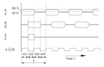
At constant rotational speed with regard to the input shaft and rotation in clockwise direction.
