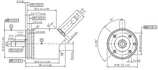
Non-tolerated dimensions according to DIN-ISO 2768-mk
