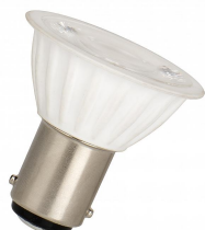
145616 LED AR37 GBF Ba15d DIM 12V 3W 280lm 830 24D
