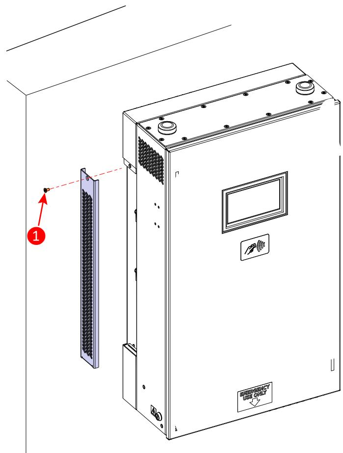
**en** The gun holder provided for the vehicle connector shall be located at a height between 500 mm and 1500 mm above ground level.
