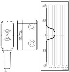
Safe switch on distance  $S_{ao}\,6\;\text{mm}$
