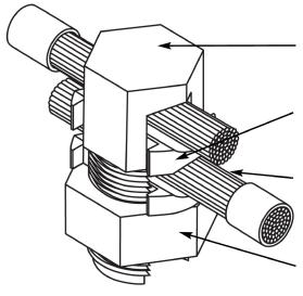
**CONNECTOR:** See that wire size is within range stamped on split bolt head.
