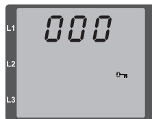
Fig. Password request If a password was set, it can be entered using buttons 1 and 2.
