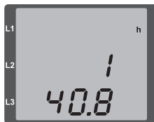
Fig. Operating hours meter of the measured value display The UMG 96RM-M shows the number 140.8 h in the operating hours meter. This corresponds to 140 hours and 80 industrial minutes. 100 industrial minutes correspond to 60 minutes. In this example, 80 industrial minutes therefore represent 48 minutes.
