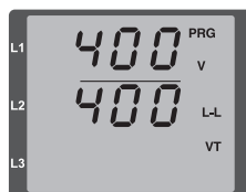
Fig. Programming mode Voltage transformer The primary and secondary currents can be changed using buttons 1 and 2 (cf. page 40).
