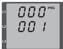
Fig. Programming mode Parameter display The individual parameters can be changed using buttons 1 and 2 (cf. page 36).
