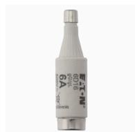
**Cartouche fusible, Basse tension, 6 A, AC 500 V, 100 kA, D1, 13.2 x 6 mm, gL/gG, IEC, lent**
