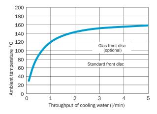
① Temperature for cooling water 20 °C, water pressure max. 5 bar
