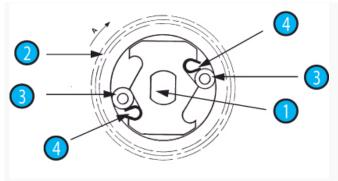
This device, situated inside the gearbox, enables the output shaft to be rotated by an external force (manual or mechanical) independently of the final wheel of the gearbox.
