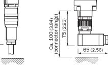
Cable sockets M26 x 11 + FE with crimp contacts
