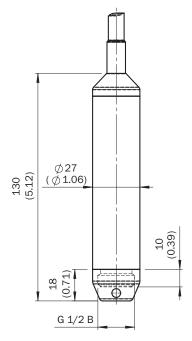
Enhanced variant with FEP cable (immersion depth up to 100 m)
