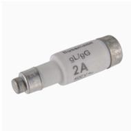
**Cartouche fusible, Basse tension, 2 A, AC 400 V, 50 kA, D01, gL/gG, IEC, lent**
