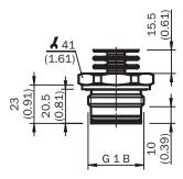
Housing with L-connector (DIN EN 175301-803 A)
