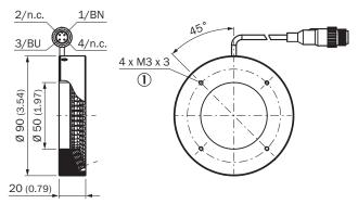
① For installation; pitch circle diameter 70 mm
