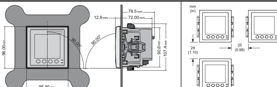
**en** Minimum clearance between mounted meters
