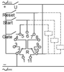
Function A : Power on Delay Relay
