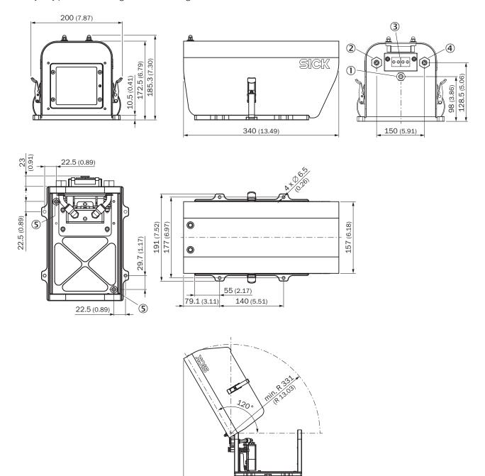
① Inlet for compressed air, push-in fitting for 10 mm connection hose, max. pressure 100 mbar (follow instructions for mounting)
