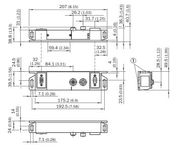
① For cylinder head screw M6 x 12
