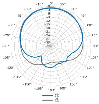
Measured antenna gain in dBic at 866.5 MHz, LHCP (left-hand circularly polarized)
