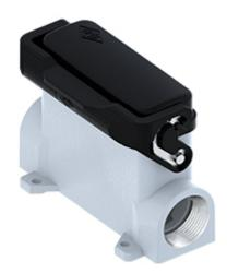
Surface mounting housing, IL-BRID series, with 1 lever, M20 cable entry, size "66.16", high construction, with SIMPLEX self-closing cover
