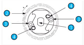
This device, situated inside the gearbox, enables the output shaft to be rotated by an external force (manual or mechanical) independently of the final wheel of the gearbox.
