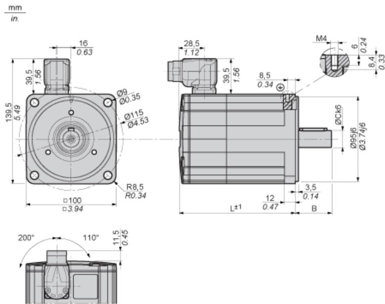
Parallel Key According to DIN 6885 A
